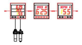
Network SPEED, DEPTH and WIND main units with DATA repeater for all functions.
