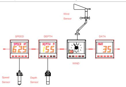
Up to a maximum of four Network DATA units maybe used in an integrated Network Instrument System, where the total number of units does not exceed twenty.
