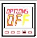
If there is no data available the Network DATA unit will display **OFF** when the **OPTIONS** key is pressed.
