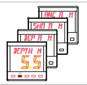
Press the **DEPTH** key to cycle through the depth options.
