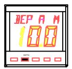
The Network DATA unit can display the depth alarm information that has been set on either Network DEPTH or Network QUAD units. It is NOT able to change the alarm values or enable/disable them. The Network DATA unit has its' own internal alarm buzzer that will sound when an alarm condition is met and transmitted over the entire Network System. It is silenced by pressing any of the five keys, in the lowest row, on any Network display unit.
