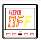
If there is no wind data the Network DATA unit will display **OFF** when the **WIND** key is pressed.
